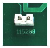
Figure 8.2: Baud rate jumper - on
