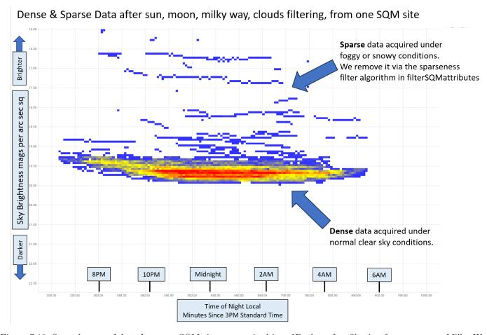
Figure 7.18: Several years of data from one SQM site summarized in a 2D plot, after filtering for sun, moon, Milky Way and clouds. Colors are proportional to the number of data points at each cell of the plot. Red represents most frequent points, blue least frequent. The goal of the sparseness filter is to remove the data points that plot away from the most dense data, to avoid bias of measurement of the clear night sky brightness. See Figure 7.19
