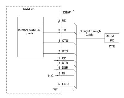
Figure 5.1: RS232 pinout
