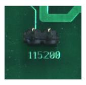
Figure 8.1: Baud rate jumper - off
