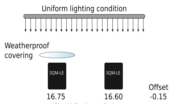
Figure 9.2: Example cover calibration
