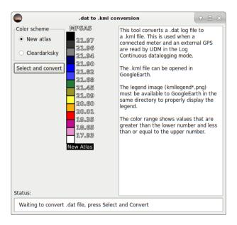
Figure 7.13: Tool: .dat to .kml
