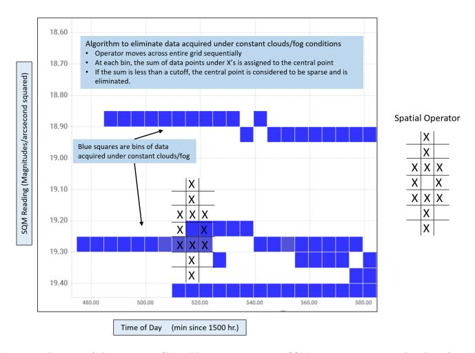
Figure 7.20: Diagram of the sparseness filter. Blue squares represent SQM measurements acquired under infrequent overcast or foggy conditions. The goal of the sparseness algorithm is to identify them for segregation into the "Sparse" output csv file.
